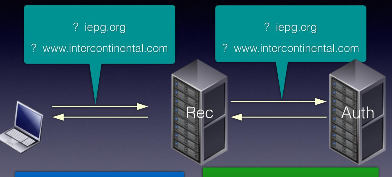
Stub Query => Rec user src address Client Subnet option (RFC7871) contains source subnet in DNS query
